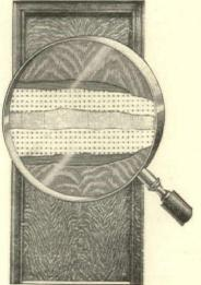
Pyrono Doors are built of finest cabinet-wood veneers applied over a nonresinous, laminated core, between which is asbestos sheathing, mechanically bonded to the core. Pyrono Doors do not expand, contract, warp, buckle nor bind in their frames under heat, making possible a tight fit that is both smokeproof and sound-proof.
