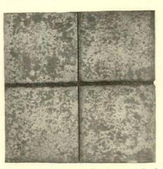
This section of concrete flooring was stained with Oak Leaf Brown. Note the color gradations and Duotone effects due to variation in the cement's lime content and density of surface.
