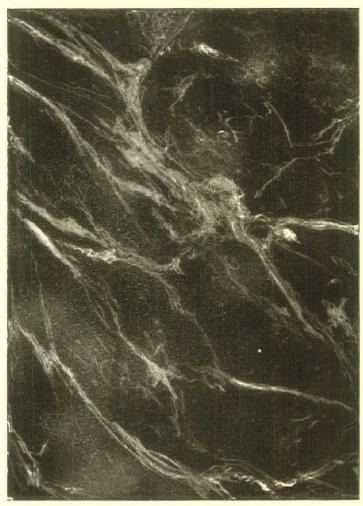
Direct photograph of a specimen of terra-cotta painted and glazed as a sample preparatory to the execution of commercial pilaster capitals above Verde antique shafts. This marble could not be carved; hence polychrome terra-cotta was a proper and unique material for this purpose.
