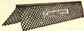
No. 1 Bead for outside corner. Pat. June 13th, 1922. Made of Tight-coat Galvanized Steel. For exterior use, with stucco, made of 16 oz. Cold Rolled Copper, also Zinc.
