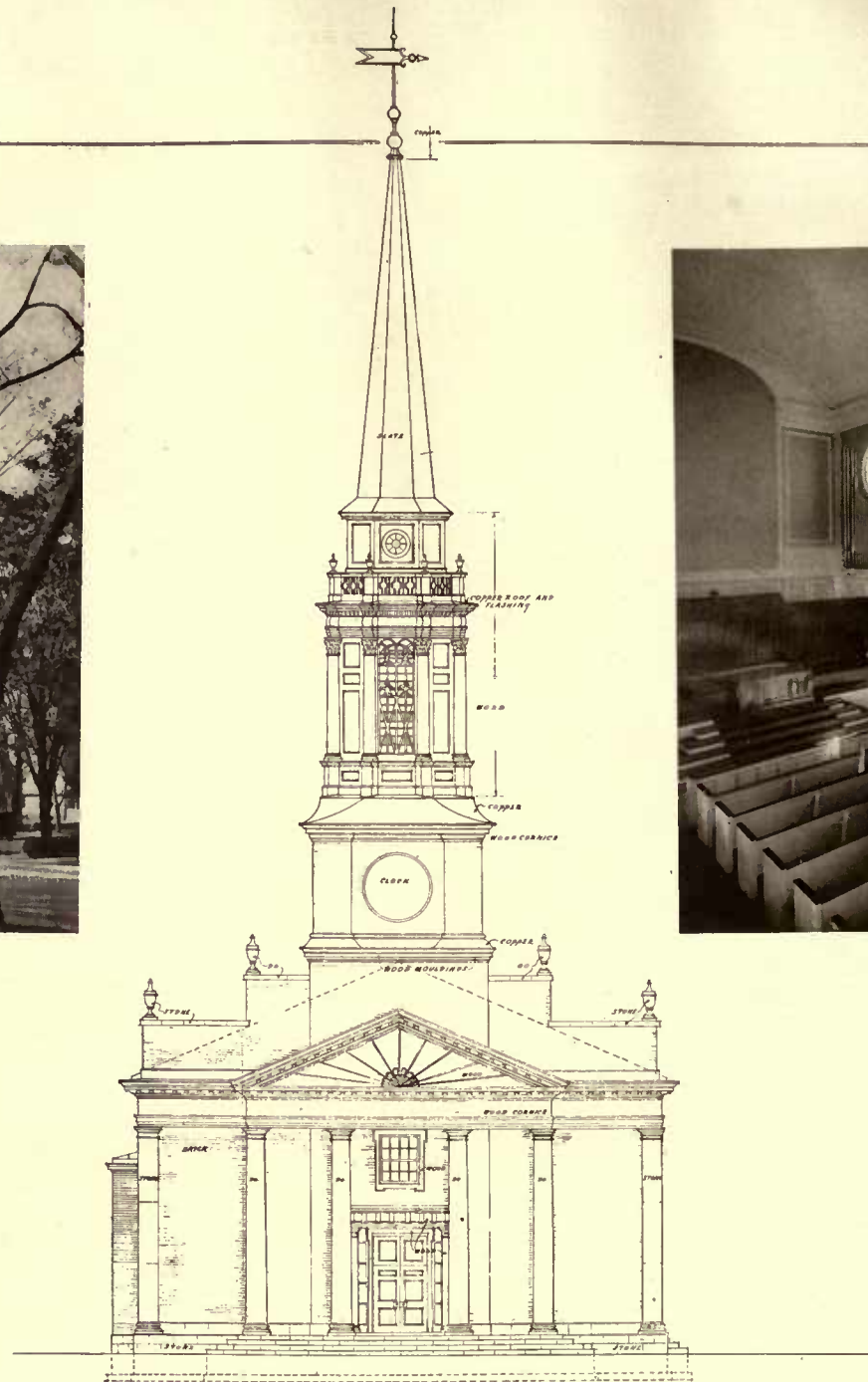
FRONT ELEVATION - CHURCH SCALE \frac{1}{4} = 1 0 CENTRAL PRESBYTERIAN CHURCH MONT CLAIR, N J
