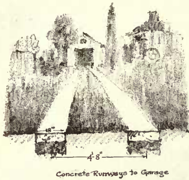
Concrete Runway to Garage
