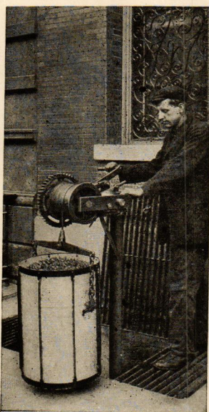
Hoisting head revolves. Can is de- posited on sidewalk without lifting.
