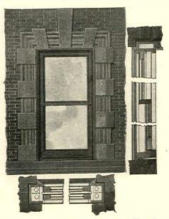
WINDOW FRAMES AND SASH, WITH PLATE OR WIRE GLASS, SHEET BRONZE OR COPPER COVERED.
