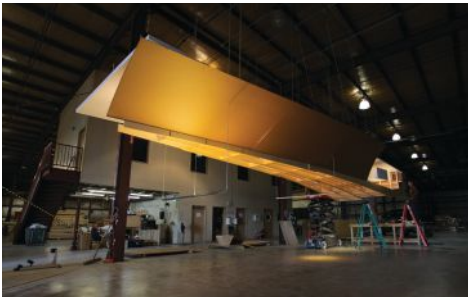
The mock-up allowed the lighting designer and the client to see how the lighting would work with the intricate wood-slat ceiling design (left). During the day, the forum is a light-filled space that welcomes the entire WashU campus (far left).
