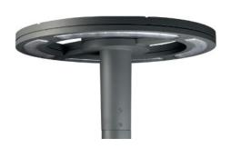
CFT500, We-ef Lighting • This post-top luminaire features a ring-shaped form factor to match a range of design styles for lighting outdoor spaces such as footpaths, parking areas, and parks. It delivers 4,536 nominal lumens but can achieve up to 8,294 lumens with 72W and 700mA forward current. It is available in 3000K and 4000K and offers symmetrical light distribution. • we-ef.com
