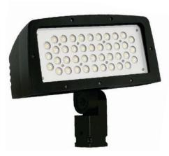
Arceos Series Floodlight, Hubbell Lighting/Spaulding Lighting • The company has added two lumen packages to its Arceos line of high-performance architectural floodlights, offering up to either 9,535 lumens or 19,368 lumens in 3000K, 4200K, or 5100K with a CRI of 80, 70, and 67, respectively. A vented housing isolates the LED module from the driver. The fixture is IP65- and IP66-rated and features a die-cast aluminum housing with seven finish options. • www.spauldinglighting.com
