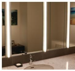
Reflections V, Dreamscape Lighting • This semi-recessed, linear LED wall luminaire is designed to illuminate bathroom vanities. Available in 3000K with a CRI of 97, the fixture is housed in an extruded aluminum frame with a curved lens that can be used alone or placed between sections of a ½"-thick mirror. Fixture lengths can be specified to meet dimensional requirements. • dreamscapelighting.com
