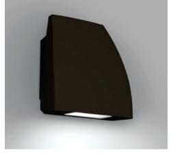
Endurance Fin Exterior LED Luminaire, WAC Lighting • This wall-mounted fixture delivers up to 2,825 lumens while consuming a maximum of 35W. Available in 3000K and 5000K, it provides 20-degree forward illumination and features a tempered prismatic glass diffuser to reduce glare. It is IP66-rated, and operates on 120V to 277V. Dimmable via zero-to-10V or electronic-low-voltage functionality. Bronze, graphite, and white finishes are available. A built-in level aids adjustments. • waclighting.com
