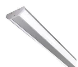
Polygon Linear LED, MaxLite • Offered in 4' and 8' lengths, each measuring 4.9" wide and 1.8" high, this low-profile luminaire is designed for parking garages and other low-bay applications requiring a linear lighting arrangement. Each fixture delivers up to 10,498 lumens in either 3500K or 5000K, while consuming 44W, 55W, or 80W; 100V-to-277V drivers provide zero-to-10V dimming capabilities. A soft-white, translucent diffuser reduces glare. • maxlite.com
