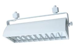
Wall Wash Biax, Elco Lighting . This trackmounted, dual-biax compact fluorescent wallwasher includes an aluminum reflector with a parabolic louver for alare control. Its housing is constructed of extruded aluminum with no exposed fasteners and measures 175/8" long and 81/4" tall. A heavy-duty mounting bracket allows for aiming with a single adjustment knob. Fitted with an integral electronic ballast, the fixture provides 2,500 or 3,600 lumens. Finishes include white or black. • elcolighting.com
