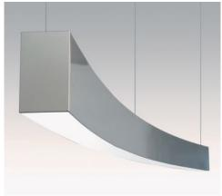
Charlotte, Birchwood Lighting • This 20'-radius curved interior luminaire can be either suspended or surface-mounted and is available in 2700K, 3000K, 3500K, or 4000K in standard, high, or custom lumen outputs. An integral electronic driver accepts 120V or 277V inputs with dimming options including zero-to-10V down to either 10% or 1%. Offered in 8' lengths with an extruded aluminum housing, frosted white or clear lens, and a satin clear anodized finish. • birchwoodlighting.com
