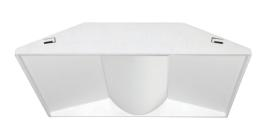
Indy X-Series, Juno Lighting Group • These basket-style LED troffers for grid ceilings are offered in 2x2, 2x4, and 1x4 models that each measure 3½" tall. Available in 3000K, 3500K, 4100K, and 5000K with a CRI of 80-plus, they deliver between 3,900 lumens and 5,500 lumens. Accepts 120V to 277V and 347V input and houses a zero-to-10V dimming driver. The fixture has a cold-rolled steel housing with a reflective white finish and built-in earthquake clips. • junolightinggroup.com
