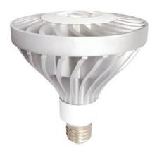
**LED NUP-PAR38, Lattice Power** • These PAR38 lamps feature GaN-based LEDs on a silicon substrate to improve light density and a thermal-pipe sink to dissipate heat without the need for active cooling. Each 27W lamp provides up to 2,000 lumens in 2700K, 3000K, 4000K, and 5000K with a CRI of 80. An alternative to 150W-maximum halogen source options in commercial spaces with high ceilings, the lamps offer 25- and 40-degree beam angles and fit an E26 base. \* latticepower.com
