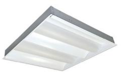
R1L/R2L Series, LaMar Lighting • Measuring less than 3" deep, this series of recessed ceiling troffers comes in 2x2, 1x4, and 2x4 sizes and is suited for use in a standard 15/16" inverted T-bar grid and shallow plenum locations. Offered in 4000K, the fixture can also be specified in 3500K and 5000K. The series provides 2,000 lumens from the 2x2 size with a CRI of 80-plus. All fixtures are designed to replace a 32W to 34W fluorescent. • lamarlighting.com
