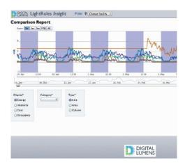
**LightRules Insight, Digital Lumens** • A cloud-based solution, LightRules Insight integrates operational and performance data from multiple facilities into a single interface for sharing within an organization. Building subsets, such as rooms, production lines, and merchandise aisles, can be called out for reporting. The application is part of the company's LightRules family, which is compatible with Internet Explorer, Firefox, Chrome, and Safari browsers. • digitallumens.com
