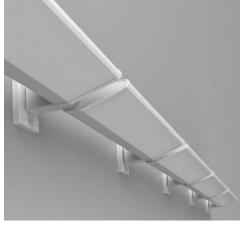
Windirect LED, Acuity Brands/Winona Lighting • This family of asymmetric indirect LED uplights is an alternative to ceramic metal halide or fluorescent fixtures for use indoors and outdoors. The forward-throw, shallow-angle luminaires offer uniform distribution and come in four profiles with outputs from 1,030 to 19,634 lumens and with a CRI of 83. Zero-to-10V dimmable. Mounting options include wall, ceiling, pendant, and basemount. • winonalighting.acuitybrands.com
