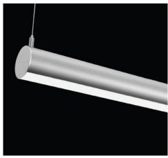
Lightplane 3 Round, Architectural Lighting Works • This 3"-diameter linear LED pendant provides 900, 1,200, or 1,500 lumens per foot and consumes 7W to 14.5W per foot in lengths of 2' to 8'. Available with tunable white or color-changing RGB LEDs as well as standard 2700K, 3000K, 3500K, or 4000K with a CRI of 80-plus. Its extruded-aluminum housing is fitted with a clear, frosted, or opal impactresistant lens. An integrated Class 2 dimming driver fits within the aluminum extrusion. • alwusa.com
