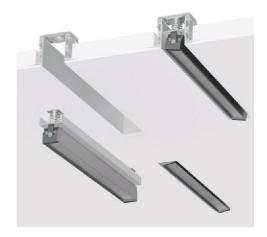
Leesti Adjustable Trimless, Archlit • This ceiling recessed trimless linear luminaire is available in 1', 2', 3', or 4' runs. Its lens features a diffusing film to create a continuous line of light. Drawing 12.5W per lumen foot, the fixture produces up to 1,400 lumens per foot in 3000K. Available for 120V or 277V inputs and dimmable using TRIAC or zero-to-10V controls, depending on the model. Powdercoat finishes include black, white, and custom colors. Damp location listed. • archlit.com
