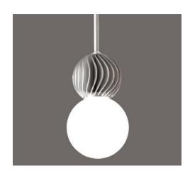
Kore LED Ambient Orb, Tegan Lighting • The Kore LED Ambient Orb is characterized by its globular aluminum-and-steel heat sink attached to a hand-blown glass sphere diffuser. It can be specified solo or with one of the company's shades. The fixture comes with a standard-output 15W module that produces 850 lumens and a high-output 38W LED module that produces 2,200 lumens. Both sources have a CRI of between 80 and 85. • teganlighting.com
