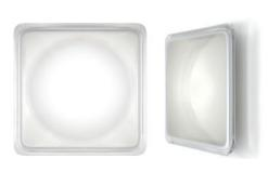
**Illusion, Luceplan** • Created by Argentine-born designer Francisco Gomez Paz, Illusion gives the impression of a sphere captured within a square—an optical effect created by the fixture's Fresnel lens and thermoplastic diffuser. The 9"-square fixture is suited for use indoors and can be mounted to the wall or ceiling. Dimmable, it is powered by a 3000K 17W LED module. • *luceplan.com*
