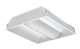
Avante LED, Acuity Brands/Lithonia Lighting • This family of direct/indirect recessed LED ceiling troffers comes in 2x2, 2x4, and 1x4 sizes for ambient indoor illumination in 3000K, 3500K, 4000K, or 5000K with a CRI of 80. The fixtures deliver lumen packages from 2,000 to 5,000. The diffusers swing down for access to the light engines and a 120V or 277V dimming driver. Metal baskets, louvers, and extruded acrylic prismatic lenses are backed with white acrylic diffusers. • lithonia.com
