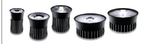
Optical Light Engines, Soraa • Compatible with many industry-standard drivers and suitable for enclosed, non-ventilated indoor and outdoor luminaires, Soraa's full-visible-spectrum GaN-on-GaN low-profile light engines produce high center-beam candlepower from narrow spot to flood. Offered in 1.5", 2", and 4" diameters, 500 and 1,000 lumens, in 2700K, 3000K, 4000K, and 5000K, and with a CRI and deep red rendering of 95.\* soraa.com
