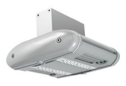
Aphos Mini Series, Eye Lighting • This 39W LED luminaire delivers 3,000 lumens in Type II, IIA, III, and V distributions, making it suitable for parking garages, canopies, warehouses, and other applications requiring bright white light. Its rugged design includes IP65-rated optics and an IP67-rated driver, while patented airflow technology draws heat away from the LED array for cooler operation. Available in 4000K or 5000K with a CRI of 70, and in five powdercoat finishes.
