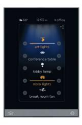
Equinox 41, Vantage • Equinox 41 is part of Vantage's Equinox family of unique user interfaces. It fits in a single-gang wall box and offers 12 widgets, including lighting, temperature, audio, video, security, timers, and shade control, in a single device. Through its 4" LCD touchscreen interface, multiple users can create personalized profiles. Ideal for high-end residential and commercial applications. • vantagecontrols.com
