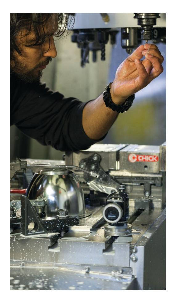
A worker changes the tool on the spindle of Edison Price's Haas Automation VF-1 vertical machining center, which CNC-mills metal parts that are used in the final assembly of the company's track fixtures, as well as supports the production of the company's track systems and R&D efforts.
