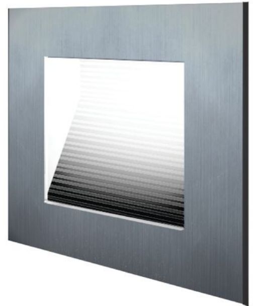
Vetrinella, Tivoli • Designed for exterior pathway or low-level interior illumination, the Vetrinella LED luminaire is outfitted with surface-mounted LEDs in 3000K, 3500K, and 4000K. The fully dimmable fixture consumes 6.5W and provides 163 lumens. Designed to fit a standard, two-gang deep-well junction box in either new or retrofit construction, the luminaire includes an integral driver and field-serviceable LED board. • tivolilighting.com
