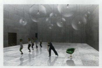
Budget restrictions meant creative lighting solutions. An early presentation drawing for the ninth floor rehearsal space (above) shows richly textured walls and a series of repetitive acrylic ball-shaped luminaires, which were eventually changed to PAR lamps in recessed sockets. Stacked like a vertical city, a section through the building (right) shows how the back-of-house spaces connect to the performance hall.
