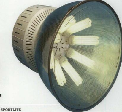
Using eight 70W lamps, the TDX architectural-grade compact fluorescent high-bay luminaire can generate 41,600 lumens, making it ideal for a variety of commercial applications. It has a lamp life of 20,000 hours, is available with a clear polycarbonate, aluminum, or a pearlescent dome, and can also be used with 120W, 85W, 60W, 57W, 42W, 32W, and 26W lamps with two-, three-, or fourlevel switching. • sportlite.com • CIRCLE 150
