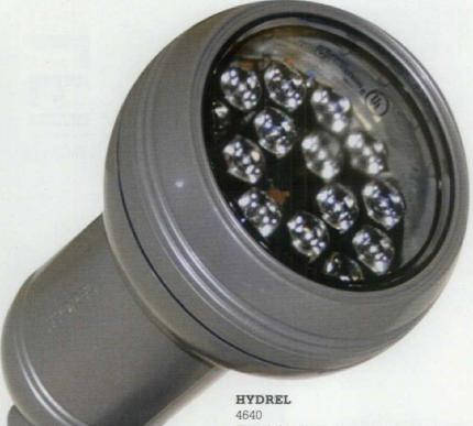
The 4640 knuckle-mount LED accent luminaire is designed with a rugged die-cast aluminum construction and an offset swivel for balance. Measuring 915/16 inches long, it has a crowned tempered-glass lens that diffuses 12W or 22W monochromatic LEDs offered in nine colors, including royal blue, warm white, and cyan. Available with wide flood, medium flood, linear spread, and spot distributions, the fixtures come in numerous (as well as custom) finishes. • hydrel.com • CIRCLE 201
