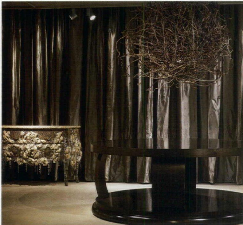
Track lighting with 20W T4 ceramic metal halide sources was selected for its flexibility, color rendering, and low wattage (above left). T5HO fluorescent wallwashers illuminate the rear walls of each furniture vignette (top right). A plan of the showroom shows the relationship of the chair "runway" and five vignette areas (above right).
