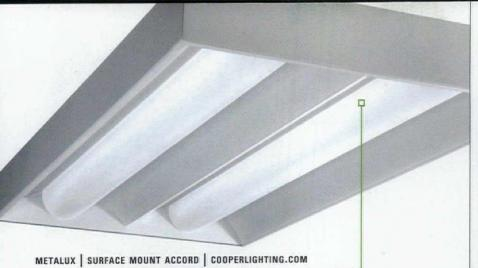
Providing comfortable illumination while eliminating surface shadows, the Surface Mount Accord improves on aesthetics and energy savings. Suitable for a variety of applications, the fixture is made from heavy-gauge cold-rolled steel painted with a matte-white polyester powder enamel finish. It accepts two T5 lamps, is available in two sizes, and contains frosted acrylic profile lenses for a soft light distribution. CIRCLE 138
