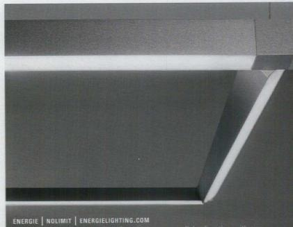
A unique lighting system that allows users to vary light direction with a simple twist of the wrist, NoLimit is slender and simple. Offering a wide range of illumination possibilities, the system is connected by a multifunction cube that joins the 4-foot lighting elements and allows them to rotate. Each lighting element contains an ultra-slim ballast and a T5 or T5HO lamp shielded by a satin diffuser. ADA-compliant wall-mount configurations also are available. CIRCLE 127
