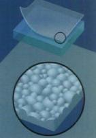
Ledalite's MesoOptics innovation speaks to advances in "thin-layer" lens technology. Tiny microstructures, 5 microns in size, are adhered to a substrate such as acrylic, polycarbonate, or glass (above). This helps remove striations and hot spots, as well as control the beam pattern (middle) or redirect the light into desired angles (top). CIRCLE 208 dlepower shape, and an additional diffuse reflector beyond the lens provides shielding.
