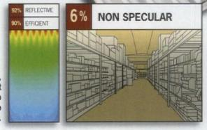
Unlike MIRO, white painted reflectors are highly diffused, offering little optical control. They have a polar light distribution unsuitable for vertical illumination. MIRO Micro Matt provides the aesthetic appearance of a white surface yet with vastly improved light controllability.
