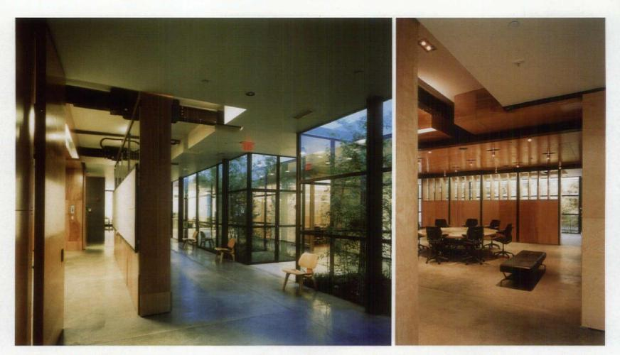
In keeping with Orange's interest in creating new work and business paradigms, the architect's responded with the "Imaginarium," a space that literally opens up with the help of custom hydraulic elevator motors installed horizontally (above left). The motors allow the side walls to pull away, transforming the center of the building from an enclosed conference room for 15 (above right) to an auditorium for 100 people. Low-voltage monopoint luminaires punch through the wood soffit of the ceiling.
