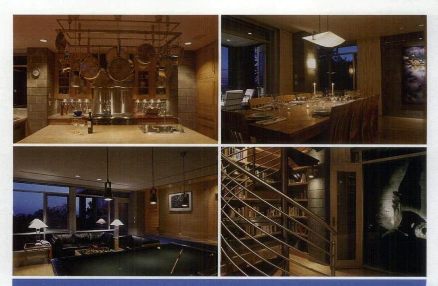
Studio Lux created a layered approach for the home, with ceiling-recessed downlights providing one level, pendants another, and table/task another throughout the 5,900-square-foot residence. All fixtures are fitted with halogen lamps to maintain a consistent color temperature throughout the house; their wattage depends on how much light is reflected and absorbed in any given space. In the master bath (below), miniaturized
