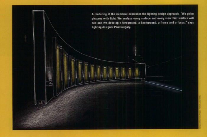
ground-recessed frosted glass that divides the monument proper from the semi-circular seating area. The channel is backlit by two rows of high-output, side-emitting fiber optics, which are, in turn, lit by four 15W metal halide illuminators—one at each end of both rows—housed in burial compartments. The white channel backing optimizes reflectance, boosting light output.
