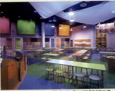
Above left: T8 fluorescent reflector strips illuminate the perimeter, creating a lavender "wrapper" for the store. Above right: Sails lighted with metal halide custom floodlights glow blue above the Studio area. Below left: Four party rooms, each painted a solid color, feature ceilings edged with LED fixtures for extra pizzazz.
