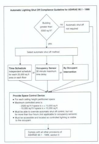
Figure 2. Controls and ASHRAE/IES 90.1-1999. Courtesy of The Watt Stopper.
