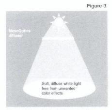
Figure 3: MesoOptics' microstructures provide fine diffusion of light without chromatic dispersion.
