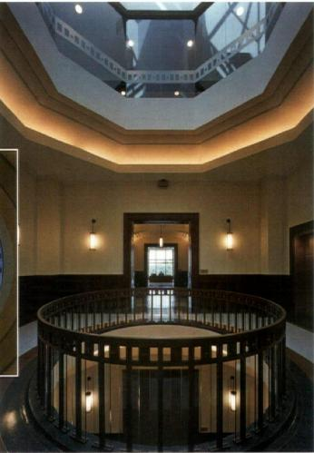
Right and inset: Natural light pours down five stories through a cupola. On the second floor, custom sconces and coves define the octagonal core beneath the cupola with additional light. The section illustrates the shaft of natural light that penetrates the five stories through the building's core beneath the cupola.
