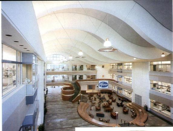
The three-story atrium features a complex lighting system that responds to the many functions of the space. The different layers of light are controlled separately for added flexibility and photocells help save energy by balancing daylight with electric light.
