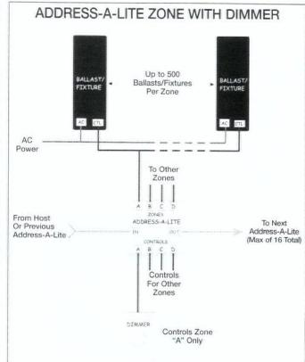
Figure 1: Easylite's Address-A-Lite system is a newcomer to the dimming/controls arena and features ballast controllers that are networked to provide a flexible mix of local and central control.
