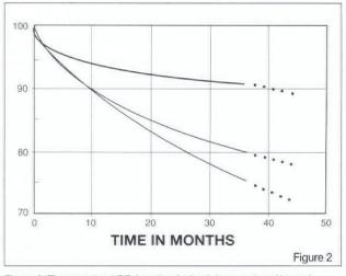
Figure 2: The tentative LDD function for both louvered and lensed fluorescent fixtures determined by the preliminary analysis of the LDD study test results (top curve). Current IESNA procedures place louvered fixtures into Maintenance Category IV and lensed fixtures into Maintenance Category V, with their LDD curves shown for comparison.
