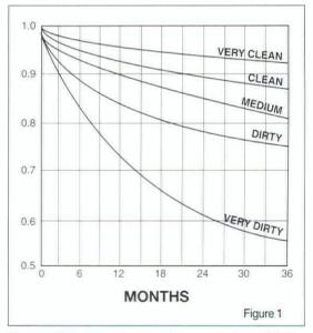
Figure 1: LDD data as it is currently presented in the IESNA Handbook. The curves estimate the amount of light reduction due to dirt accumulation on fixture surfaces.
