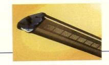
Venza LP from **Ledalite** is offered in a one- or two-T8-lamp version and a T5/HO version. Venza offers semi-indirect, indirect and wallmounted distributions and is available in in 4-ft., 8-ft. and 12-ft. lengths. Housing is die-formed, 20-gauge cold-rolled steel. Finish is standard white or Techspace natural steel metallic powder coat. Translucent endcaps come in seven colors. UL-listed. **Circle No. 167**
