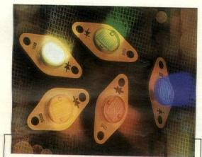
Opto Technology's Shark Series of high-flux LED illuminators offers five standard colors: blue (470 nm), green (530 nm), amber (590 nm), red (630 nm) and white. Typical brightness from Red Shark is 55 lumens. All models incorporate 50 LEDs die-mounted to a BeO substrate that is attached to a TO-66 power package. The thermal packaging allows the series to run at high currents and ensures extended reliability. Units can be operated in continuous or pulse-mode illumination. Circle No. 204
