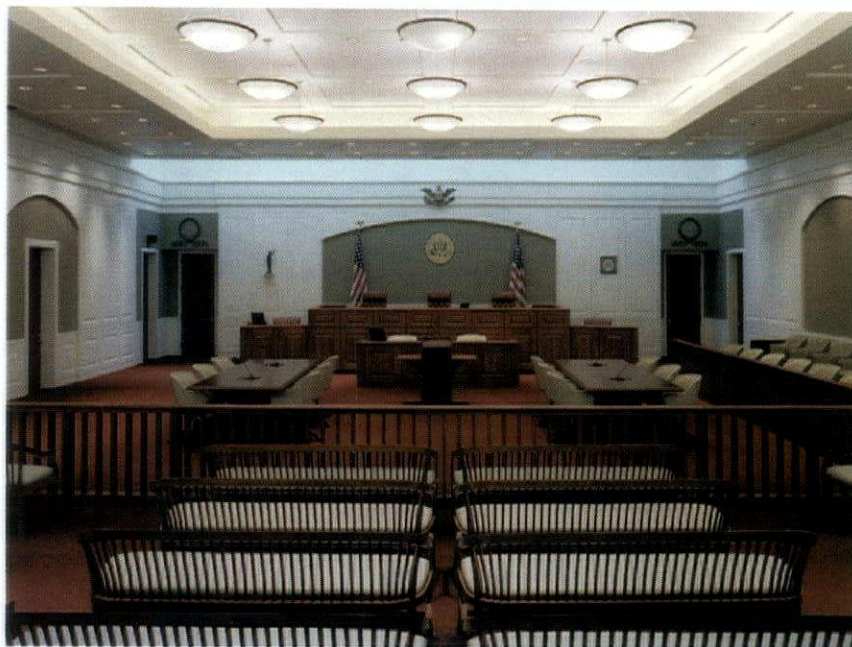
Downlights and wall washers are used in all of the courtrooms to provide ambient and task lighting and to accentuate the spaces' architectural forms and traditional finishes.
