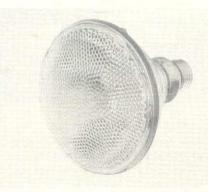
GE Lighting now offers the XL Ultra Life version of its HIR PAR lamp, which offers a life of 6,000 hours, three times longer than a standard halogen PAR lamp. The HIR XL Ultra Life PAR lamp is available in 45W, 55W and 90W as well as 12- and 40-degree beamspreads. Circle No. 236
