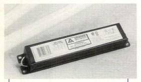
Advance Transformer Co. has expanded its Centium line of electronic fluorescent ballasts with new "small can" designs for one, two, three and four-lamp operation of F17T8, F25T8 and F32T8 rapid start lamps on both 120V and 277V systems. The ballasts' new reduced size dimensions are 1.7 in. wide, 1.18 in. high and 9.5 in. long, resulting in a reduction of about 5/8 in. in width and 1/3 in. in height compared to standard-sized ballasts. Circle No. 234
