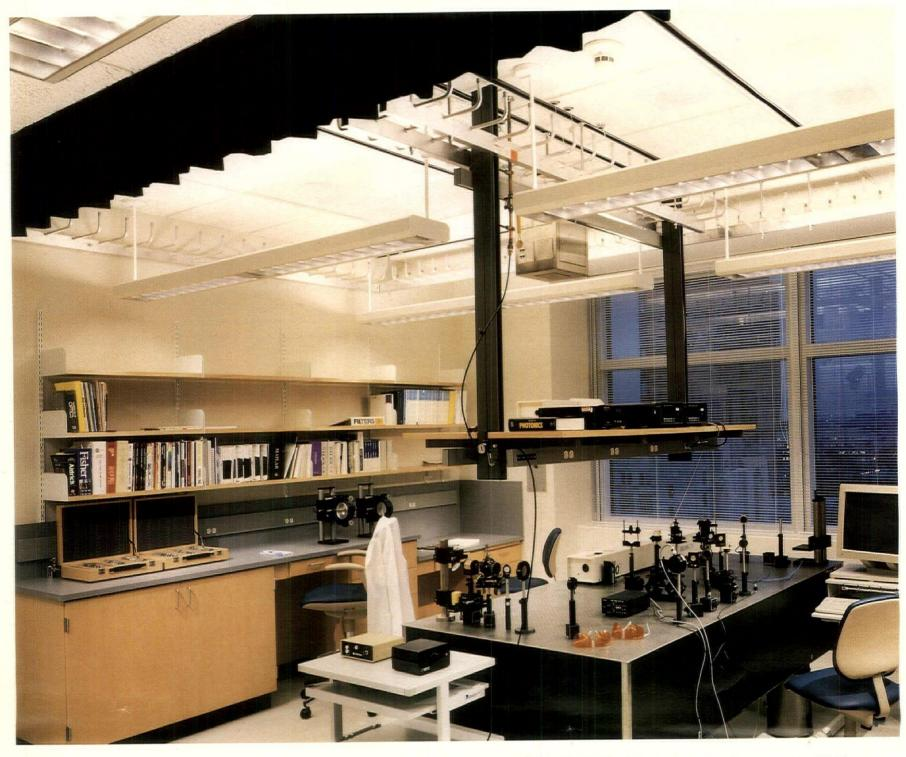
ABOVE: LAB SPACES EMPLOY DIRECT/INDIRECT FLUORESCENT FIXTURES TO ILLUMINATE THE SPACE, WHICH IS DESIGNED FOR RESEARCH ACTIVITIES. THE CENTER IS DEDICATED TO EXPLORING THE USE OF LIGHT IN TECHNOLOGY, SUCH AS LASERS, LEDS AND SCANNERS.
