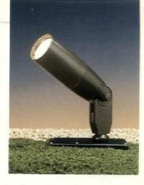
horizontal adjustment and fastening. Coronado is available in 35W PAR20 (#720), 35W and 70W PAR 30 (#730) and 70W and 100W PAR38 (#740). The series is constructed of both cast and machined corrosion-resistant aluminum alloy with a tempered glass lens secured in place by a high-temperature adhesive. All hardware is stainless steel. Standard finishes are Architectural Bronze, Black, White, Verde and City Silver. Other colors and plated finishes can be custom ordered. Circle No. 66
