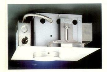
Edison Price's Anglux AR/4 is an adjustable accent light used to highlight art in the Red Mountain Residence. Anglux AR/4 has a 4-in. aperture and uses a 12V quartz halogen AR70 lamp. A conical reflector design minimizes aperture brightness. The fixture has a 0- to 35-degree angular lamp adjustment with a 358-degree horizontal rotation. Recess depth is  $6^{3}$ /<sub>4</sub> in. Three kinds of lenses, a UV filter and six glass color filters are available. Circle No. 50
