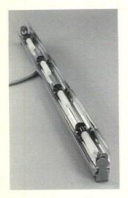
Tucked in the clerestory, Elliptipar's Style 301 linear incandescent fixture illuminates a soffit to create the illusion of a floating ceiling. Constructed of extruded high purity aluminum with a clear anodized specular finish, reflectors can be mounted in a continuous row; joiner screws lock reflectors together and allow all in the row to be aimed together. Mill finished aluminum L-shaped mounting brackets can be base-, wall- or ceilingmounted. Circle No. 56
