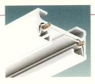
Lighting the display niches, **Juno Lighting's** One-Circuit Trac-Master System, T8-WH, offers One-Circuit Trac-Master sections that can be surface-mounted or suspended from ceilings with pendant accessories. One-Circuit Trac sections feature an extruded aluminum channel, General Electric Noryl 265 insulator, debossed polarity line, No. 12 solid copper conductors and concealed wireway on top of the Trac section. **Circle No. 77**
