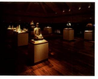
In lighting the mezzanine space, the lighting solution called for general ambiance with focused light on individual displays. The lighting designers used high-angle AR 4-, 8- and 25-degree focused light. Linear and bilateral spread lenses and hex louvers were selected for beam and glare control.
