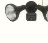
Lighting's Infrared Motion Activated Floodlights series features an adjustable infrared sensor mounted on the fixture to detect motion in a 110degree area up to 80 ft. to the front and sides. A 180-degree/65 ft. deep detection area is also available. A dusk-to-dawn photocell automatically deactivates the detector during daylight. A manual override allows for remote setting. 150W twin PAR units are available in standard wall boxes. UL-Listed. Circle No. 170
