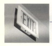
efficient exit signage constructed of lightweight injection-molded thermoplastic with a polycarbonate panel for even illumination. Exit signs can be specified in wall-, sideor ceiling-mounted models and use energy-efficient LEDs or cold cathode light sources. AC-only and selfpowered/emergency-operation models are available. Self-powered models use a long-life nickel cadmium battery. UL-listed. Circle No. 81
