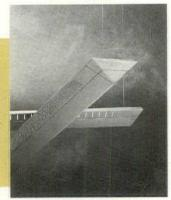
Readi Cove from **Tivoli Industries** uses compact fluorescent and incandescent lamps in straight or end-to-end and side-by-side lamp configurations. Extruded aluminum pre-wired channels snap into modular formed steel housings in modules that connect to fit various application requirements. Fascias may be specified in different styles and finishes. Integral ballasts are available in
