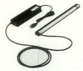
Häfele's sub-miniature fluorescent light features a flicker-free electronic ballast specially designed to operate sub-miniature fluorescent lamps. The ballast uses Quicksense technology, in which the patented circuitry in the ballast shuts down the system when the lamp reaches the end of its life. The lamps have pure tri-phosphor coating, which provides a CRI rating of 80. UL-listed. Circle No. 206
