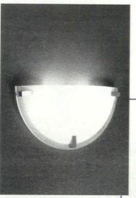
Advent Lighting's AS3046 wall sconce features luminous opal acrylic lens and a 1/2-in. thick Duramorphos acrylic half ring. The wall sconce mounts to a standard 4-in. junction box and measures 20 in. x 10 in. Lamping options include two 40W T10 incandescent or two 13W twin-tube bi-pin compact fluorescent lamps. AS3046 protrudes 4 in. and is ADAcompliant. All ballasts are electromagnetic. Various finishes are available. UL-listed. Circle No. 123
