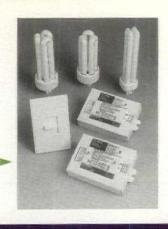
Originally introduced with a ballast for 32W, 4-pin compact fluorescent lamps, Lutron Electronics' Tu-Wire line now includes ballasts for both 26W, 4-pin triple and quad-tube compact fluorescent lamps. Tu-Wire electronic fluorescent dimming ballasts use only two wires for power and control and provide architectural dimming for compact fluorescent lamps down to five percent light.
