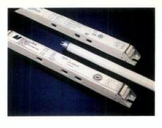
for use with 14W, 21W and 28W lamps. The ballasts have a high power factor; feature less than 20 percent THD; feature a shutdown circuit to turn off the ballast at the end of lamp life; preheat the cathodes; protect against overvoltage; feature poke-in wire trap connections; and come in a small size (3/4 in. height). UL pending. Circle No. 103
