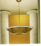
disk with one side frosted. Four machined aluminum grip blocks with a brush finish support the green disk, while gripping the spun dome. A single aluminum center stem, also with a brush finish, completes the product. The light source is a 6-26W quad compact fluorescent using electronic integrally mounted ballasts.
