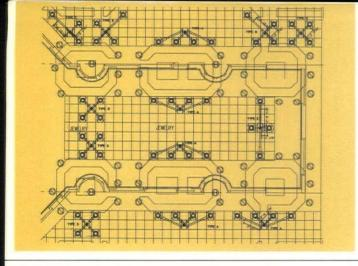
AT JCPENNEY, THE MULTI-BEAM SYSTEM REPLACED RECESSED AND TRACK-MOUNTED HALOGEN PAR ACCENT LIGHTING FIXTURES ON A ONE-TO-ONE BASIS. (CIRCLES REPRESENT FIXTURES; THE CONNECTING LINES LEAD TO THE LUMENOSITER, WHICH HOUSES THE LAMP.)
