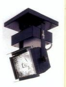
rendering (82-85 CRI) and an average life of 6,000 hours. A wide beam pattern is controlled by easy-fitting barndoors, louvers and filters. The MC420 is equipped with tempered safety glass and offers numerous mounting options.
