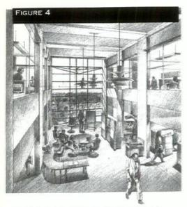
• A 9 ft. 6 in. interior ceiling height within a 13 ft. floor-to-floor height to permit the design of an indirect lighting system and maximize the depth of daylight penetration.
