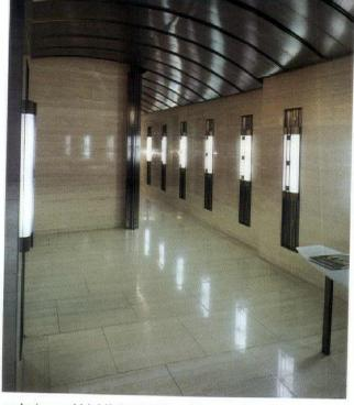
and trim, and highlighted with architectural detail, produces a deep, rich ambiance. Therefore, it had been imperative to conceal the lamps and use glare-resistant fixtures that would gently and sufficiently light the space, while not detracting from the general atmosphere.
