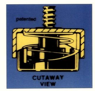
D on't let the wobbles ruin your new table's debut. ON THE LEVEL's Superlevel<sup>TM</sup> Table Glides automatically adjust to a floor's surface every time a table is moved. The secret is a double cam and spring mechanism. Superlevel's stainless steel spring is housed in a super-tough nylon body that won't damage floors or carpets. For further information contact: On The Level Co., Inc.: 800-4-GLIDES.
