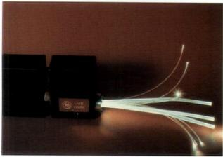
Not only is the Light Engine able to introduce the largest amount of light into very small light guides or fibers (viz. less than 10mm diameter) of any of the incandescent or metal halide illuminators on the market, but because of the low wattage of the lamps, it is possible to operate the engine in an enclosure without a cooling fan. The metal halide source gives it a long average life. In addition, instant light and relight also makes it different from other metal halide illuminators.
