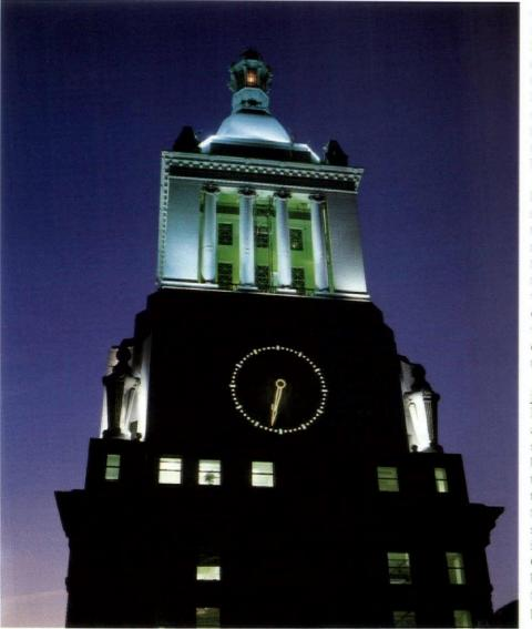
with two fiber bundles. Each 45strand bundle is lighted with a separate Light Engine. Each hour hand is illuminated with one engine and one bundle of fibers that also replace incandescent lamps. An optic at each fiber strand end spreads the light via refraction and total internal reflection so the hands appear bright from every angle of view.
