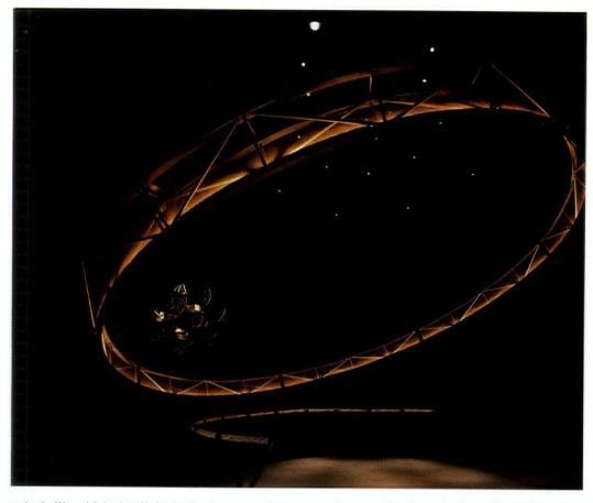
atrical ellipsoidals that light the background with the HQI sources that light the foreground was difficult. After much trial and error with color media, paint retouching of the background under the light source helped resolve the issue.
