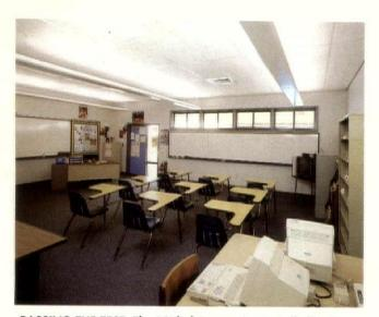
PASSING THE TEST: The LCI lighting system installed in these classrooms provides indirect lighting while maintaining good vertical and horizontal illumination, allowing students to work at their desks or on computers without glare or shadow.
