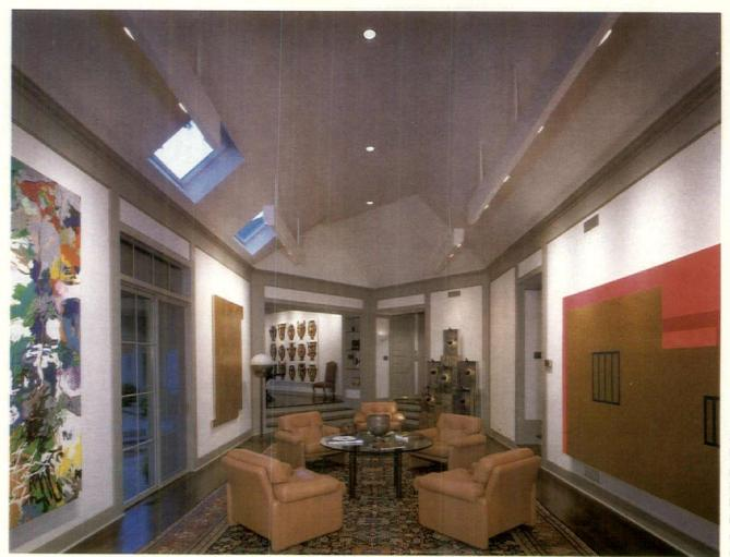
BAFFLED SYSTEM: Installed behind the baffles, low-voltage PAR 36 fixtures focus on details (below), while PAR 38s wash the walls (below right). ARTISTIC APPROACH: The lighting system for this private gallery (left) illuminates the interior, highlights the artwork and complements the clean lines of the architecture.
