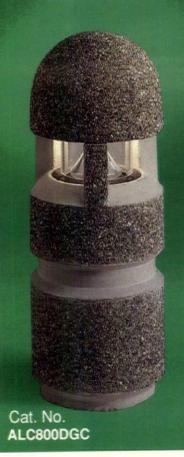
DURABLE LIGHTING - Dome Top Bollards constructed of reinforced precast concrete with a cast aluminum grill and an inner high impact acrylic diffuser encloses a variety of H.I.D. lighting. Choose from (3) standard mounting heights and (2) textured finishes. Concrete colors and ceramic tiles are available.
