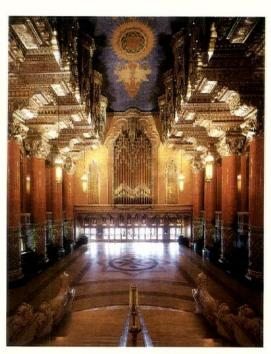
A grand vista unfolds at the center entrance of the second balcony in the theater. The proscenium front, bejewelled and mystical, has been substantially illuminated from the rail lights on the first balcony. The 500-watt, PAR 56 spots have been added, aimed upward, and positioned on an angle to eliminate the ever-present glare potential, which occurs when lights are aimed directly at gilded surfaces.
