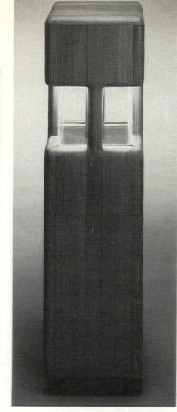
WOODFORM'S MODEL 4515-37 REDWOOD OUT-DOOR LIGHT FIXTURE accommodates low-wattage metal halide lamps. Series 4000 fixtures utilize performance optics and a concealed reflector assembly to maximize light distribution and minimize glare. There are 16 styles available in heights ranging from 37 inches to 84 inches. Woodform, Inc., Portland, OR. CIRCLE 34
