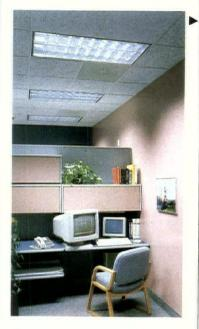
THE OPTIMAX LIGHT CONTROL SYSTEM FROM LITHONIA LIGHTING is a fluorescent lighting system that eliminates glare, and provides appropriate levels of general illumination for tasks. This recessed parabolic, with a specular aluminum louver designed to direct light away from glare-producing angles, provides a uniform level of 70 maintained footcandles of illumination. This system is available in 2-foot x 4foot and 2-foot x 2-foot models. Lithonia Lighting, Conyers, GA. CIRCLE 48
