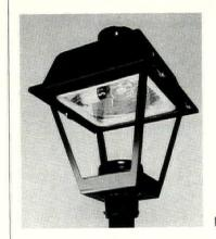
GE LIGHTING SYSTEMS' HUDSON LUMINAIRE provides cutoff optics for roadways and many other outdoor facilities. The clear glass lens and reflector are mounted inside the hinged canopy. The fixture uses HPS lamps of 50 to 150 watts. Decorative poles are available. General Electric Co., Hendersonville, NC. CIRCLE 45
