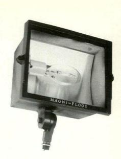
MAGNI-FLOOD'S MINI-FLOODLIGHT with a multi-voltage ballast utilizes HID light sources and measures 10 inches × 7 inches × 6 inches. The miniflood is available in 35-watt to 150watt high-pressure sodium, 50watt to 100-watt mercury vapor, and 100-watt metal halide. Magni-Flood, Inc., West Babylon, NY. *Circle No. 55 on product card.*
