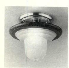
**Ceiling-mounted luminaire** Fredrick Ramond offers the model 337-CM ceiling-mounted luminaire from its Geo Collection. It has an etched glass diffuser, a disk of marblelike white or granitelike black Corian, a synthetic stone, and metal accents in polished brass, antique patina, and brushed steel. The luminaire accepts a 100-watt A lamp. Fredrick Ramond Inc., Cerritos, CA.
