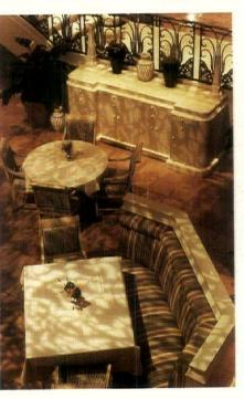
At night, lights are turned up, and the dramatic lighting comes to life. Theatrical spotlights, mounted on beams at the third-floor level over the atrium, project leaf patterns down to the restaurant floor below. The patterns are made with leaf-shaped steel templates inside the fixtures. Leibow describes the effect as "a natural feeling, almost of sunlight coming through the trees."
