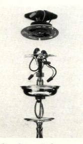
Ceiling-fixture jack Wiremold's Wire Light ceiling-fixture jack is a two-piece system with a mounting plate and a jack. Installation involves inserting the jack into a mounting plate, pushing up, and twisting it to make electrical and mechanical connections. The pieces disconnect easily for removal, relamping, or cleaning. The Wiremold Company, West Hartford, CT.
