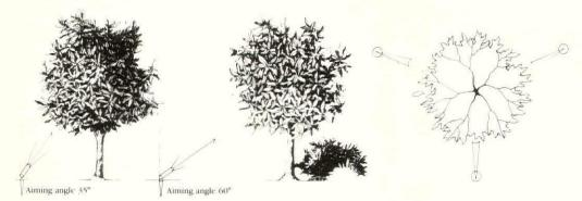
Trees with dense, rounded forms, such as the southern magnolia (Magnolia grandiflora), require multiple fixtures outside the canopy. When the tree will be viewed at close range (when it's near a walkway, for example), from several sides, and/or if no object will block a view of the fixture face, use 35 degrees from vertical as the maximum aiming angle. If something blocks the view of the fixture face, the angle can be increased to as much as 60 degrees.
