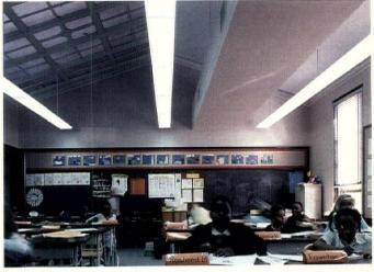
Classrooms at Cook School have gabled roofs and northfacing double-glazed skylights. The heavy, pebbled glass of the interior skylight diffuses direct sunlight and minimizes glare. The architects added three rows of pendant-mounted fluorescent luminaires with wraparound prismatic lenses to reduce brightness contrasts between the skylight and the rest of the ceiling.
