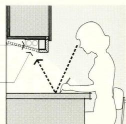
Small-cell louvers installed at an angle underneath the lamps shield the reflected lamp images, which reduces the lighting level but substantially increases task visibility.
