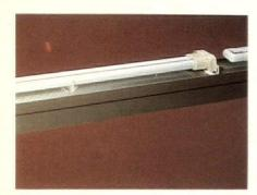
Compact fluorescent strip A compact fluorescent light strip from Norbert Belfer has an extruded aluminum continuous raceway in factory-mitered runs and custom lengths. The quiet selfstarting ballast is housed in the raceway; lift-up sockets allow for easy relamping. Three models are available to accommodate lamps from 18 to 39 watts. Norbert Belfer Lighting, Ocean, NJ.
