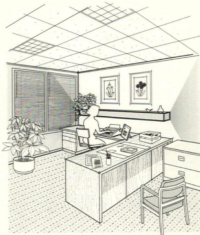
Lighted low wall brackets provide light with a soft diffused quality and both indirect general lighting and direct task illumination.
