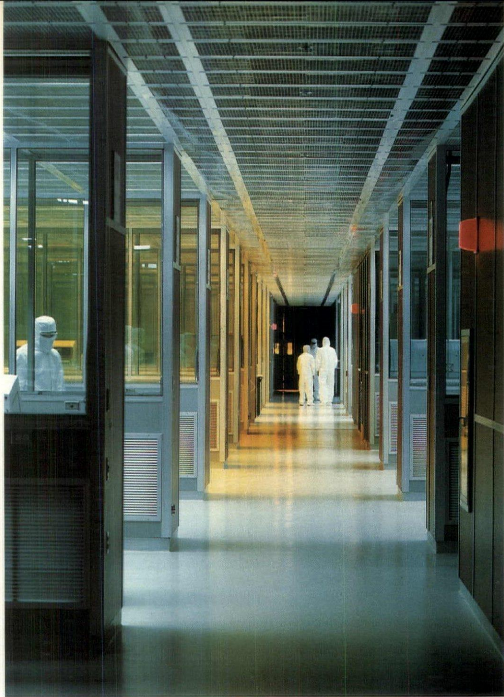
The work bays for photolithography have yellow darkroom lighting, others have white light.
