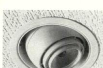
■ Recessed low-voltage fixture The Recessed Orb II from the Alesco line of Sylvan Designs is a miniature recessed luminaire for 20- and 50-watt halogen lamps. It measures less than 6 inches in diameter, including trim ring. The luminaire can be rotated 360 degrees horizontally, adjusted as much as 30 degrees from vertical, and locked in place. Sylvan Designs, Inc., Northridge, CA. Circle 78
