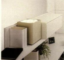
■ Portable HID uplights SPI Lighting's SPD portable HID indirect luminaires are 14½-inch-high cubes with rounded corners and either rubber feet (for flat surfaces) or mounting brackets (for office panels). They have multifaceted specular reflectors for symmetrical or asymmetrical distribution. SPI Lighting Inc., Mequon, WI. Circle 114
