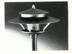
■ Low-voltage outdoor lighting The Footliter from Nightscaping produces a glare-free circle of low-level illumination 14 feet in diameter. The manufacturer notes that a unique electrostatic process for bonding a powder coating to the all-metal fixture increases its resistance to impact, weathering, and air pollutants and extends its life to 10 years. The spike-mounted luminaire is 10 inches high and comes with a 12-volt, 12.3-watt LL93 lamp. Nightscaping, division of Loran, Inc., Redlands, CA.
