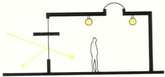
Tinted or reflective window glazing will reduce glare only if the space is lighted by other sources, such as electric lights or skylights.
