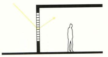
Light-directing glass blocks have built-in prisms that can be used to refract light toward the ceiling.
