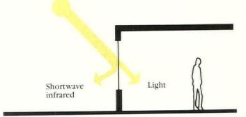
The ideal selectively transmitting glazing would reflect all of the sun's infrared radiation and would allow the visible light to pass through.
