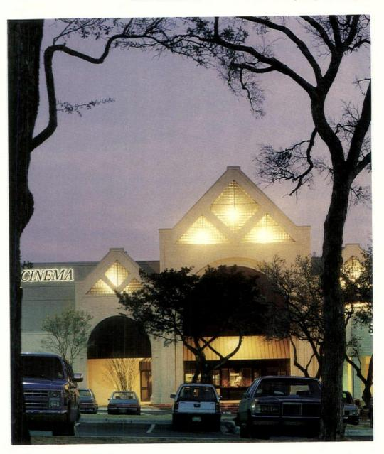
Nighttime view of the cinema showing ticket vestibule and deep arcades covered with canopies, designed to prevent direct light from hitting the cinema's exterior glass wall.
