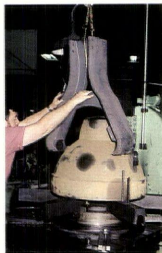
At the machine shop (left), milling machines flatten rough surfaces where metal parts must fit together or where rubber gaskets will be installed. Drilling and threading for pins and connectors is completed. A machinist test fits a yoke casting
