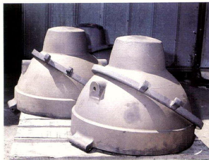
to one of the fixture housings (center left). After being sandblasted, degreased, hot-dip galvanized, and painted, these fixture housings (right) will be installed at the bridge.
