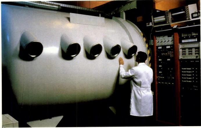
A vacuum coating chamber used in the manufacture of low-emissivity glass.
