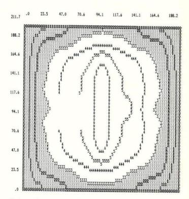
Dot matrix printout from a Lumen-Point calculation for a 200-foot by 200-foot parking lot. Left: borizontal illuminance in footcandles, printed to scale with various grid statistics. Right: borizontal lumens per unit area; criteria: less than 3, shaded; greater than 3, clear.
