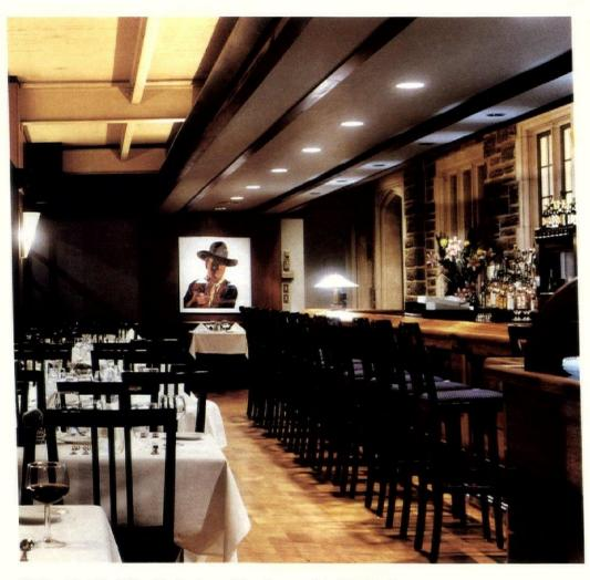
Wall washers heighten the texture of the stone wall behind the bar.
