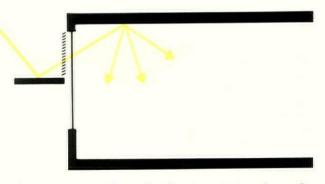
Light shelves act as overhangs for the view windows beneath; louvers can be used to avoid glare caused by the glazing above the light shelf.
