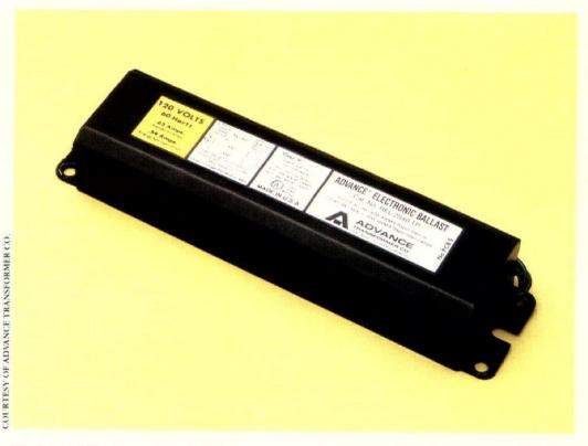
The label of this electronic ballast lists electrical specifications, compatible lamps, thermal protection (Class P) and sound ratings, and minimum starting temperatures. The second panel from the left shows a wiring diagram and details installation requirements.
