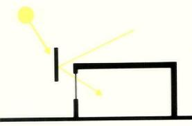
A vertical panel can block direct sunlight while reflecting diffuse skylight.
