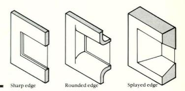
Excessive contrast between a window and a wall can be minimized by splaying or rounding the inside edges.
