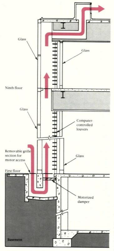
The Hooker Office Building, Niagara Falls, New York, uses computer-controlled louvers to regulate the light and heat entering the building.
