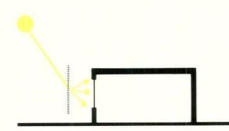
Sunlight can be filtered and softened by trees or by such devices as trellises and screens.
