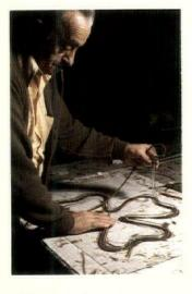
A blow tube keeps the glass from collapsing during sharp bends.
