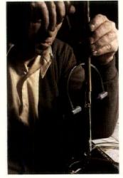
Attaching an electrode with a hand torch and an electrode holder.
