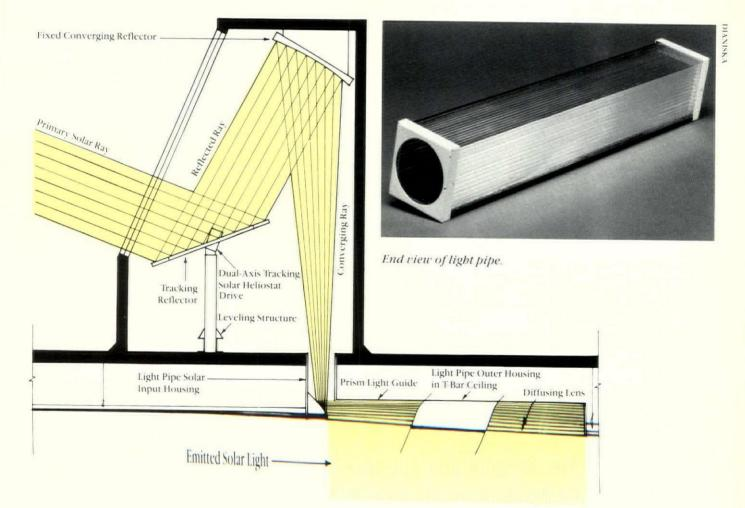
Schematic of the solar light pipe at Victoria Park Place.
