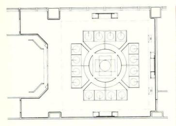
Sixteen sandblasted glass disks rest on bronze brackets along the perimeter of the five-part lighting structure. Each of the four lacquered-wood elements and the central reflector assembly are independently suspended. Lacquered display porticos accent the boardroom's walls.
