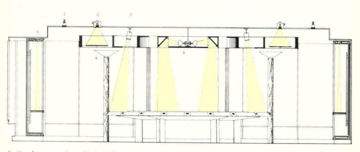
Section shows mountings of (1) incandescent downlights, (2) low-voltage MR 16 downlights, (3) low-voltage PAR 36 spotlights, (4) tungsten halogen wall washers mounted within the lighting structure and in torcheres, and (5) low-voltage incandescent floodlights.
