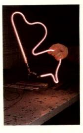
Filled with neon, sealed, and lit, the new lamp appears pinkisb. As it ages, its color deepens to orange-red.
