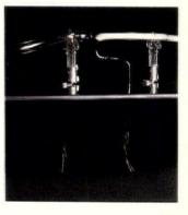
Detail of an unfinisbed neon sculpture shows clear and coated glass on a plastic mounting board. Note blackout paint, glass tube supports in metal bases, copper tie wire, and electrodes passing through boles in surface.
