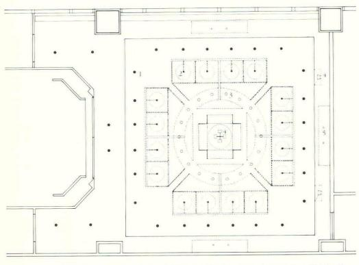
A central dimmer system adjusts light levels by controlling (1) incandescent downlights, (2) low-voltage MR 16 downlights, (3) low-voltage PAR 36 spotlights, (4) tungsten halogen wall washers, and (5) low-voltage incandescent floodlights.
