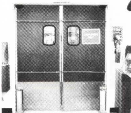
SCP 8: A Solid Core decor door. Illustrated door has 18" high Base Plates and Edge Trim (18 gauge Stainless Steel). Decorative High Pressure Plastic Laminate above Base Plates to top of door both sides. For Food Service and other areas where Solid Core Decor doors desired. Write for other models and options.
