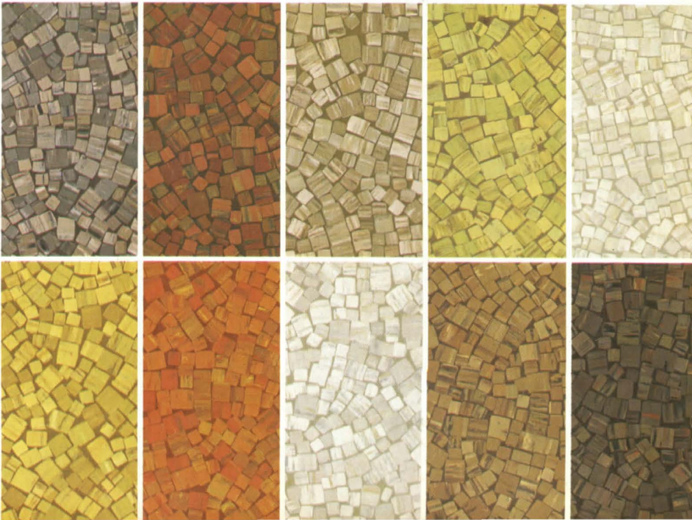
Inlaid construction —color and design go through the wear layer. Sample has been milled down in 10-mil increments.
