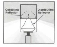
The Pericline Optical System.Light is projected outward by the patented dual reflector train in a highly efficient, gradated beam. Maximum beam intensity strikes the ground  $2\frac{1}{2}$  to 3 times the mounting height from the pole. Beam intensities nearer to the pole are gradually reduced providing uniform levels of high illumination across wide areas.
