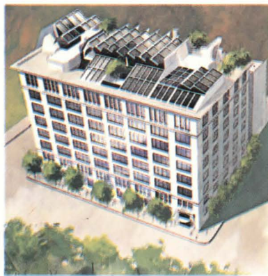
Printing House, New York City. Recycles an obsolete industrial building to create unique urban style housing. A vertical heat pump provides heating and cooling. Solar panels provide energy for domestic hot water. All insulation standards are upgraded. All windows are \frac{3}{8} -inch insulating glass.
