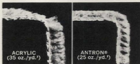
Abrasion test on simulated stair edges shows pile wear in level-loop carpets after equal exposure.
