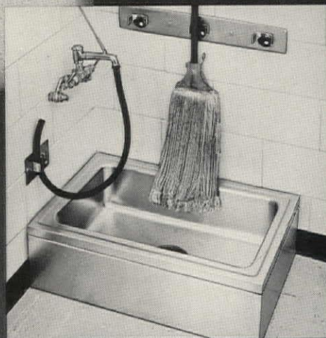
Floor Service Sink Model EFS-2523. Designed for maximum convenience as a mop sink. Standard fitting LK-43 stainless dome strainer for caulking 3" I.P.S. Additional equipment available: LK-401 faucet, LK-402 hose, LK-403 3-station mop holder and LK-404 hose hanger.
