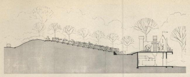
Brenau College steam plant is located in a ravine and acts as a dam to hold back earth, at the same time providing a natural stage for an amphitheater. All exposed materials are muted to harmonize with the color of the concrete. Woodmen of the World State Service center (right), on a hill, doubles as a landmark for the Gainesville area.
