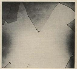
Simulated accident demonstrates that muntin bar aggravates injury rather than preventing it. The crossbar stops the body, but the head pitches forward, just as when the motorist slams on the brakes in a panic stop. When ordinary annealed glass shatters, sharp, jagged edges are left. Tempered glass (bottom right), which is five times stronger, on the other hand, only breaks under severe impact, crumbling into small pieces.
