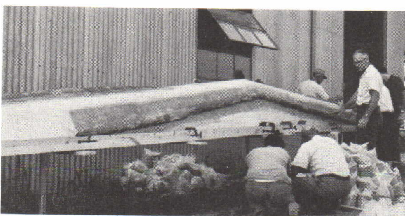
First test unit with stiffening ribs grafted on
